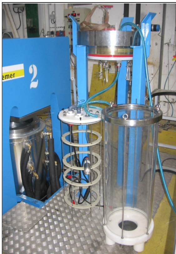
FIGURE 3: THE HYPERBARIC CHAMBER AND ELEMENTS OF THE CONTAINMENT OF THE TEST MEDIUM ALLOWING SENSORS TO BE SUBJECTED TO HIGH HYDROSTATIC PRESSURES AND A REGULATED TEMPERATURE BETWEEN 4 AND 20 °C.
