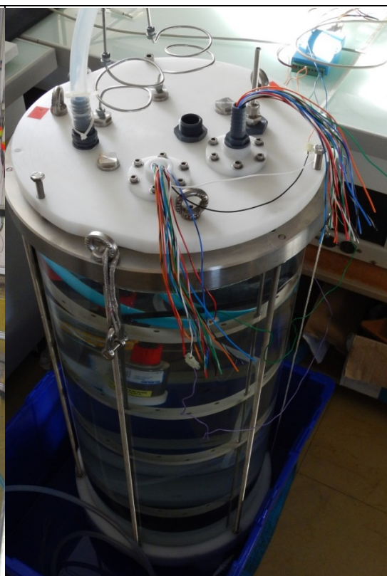
FIGURE 4: THE CONTAINMENT CHAMBER OF THE TEST MEDIUM WITH THE COVER PROVIDED WITH ELECTRICAL AND FLUID PASSAGES FOR CONNECTION TO THE OUTSIDE OF THE HYPERBARIC CHAMBER.
