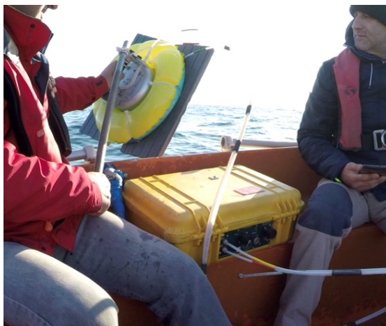
Figure 25: customized accumulation chamber and fluxmeter equipment during on-field measurement
