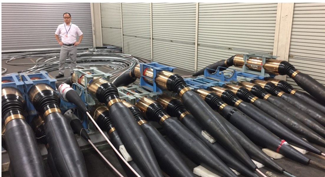
Figure 6 : Repeater stack during factory testing (from Lentz and Howe, oceans'18)
