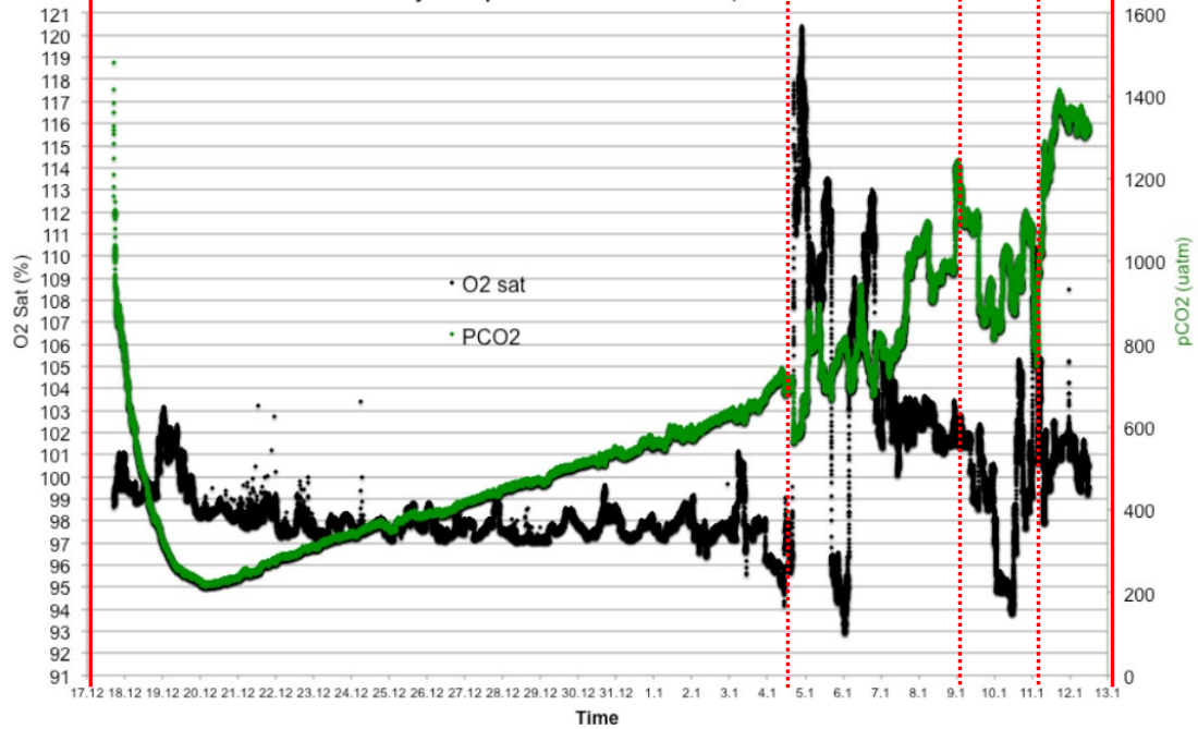
Figure 4. Reference pCO 2 data from the GO underway pCO 2 system (A) and the Aanderaa pCO 2 optode (B, green symbols) as recorded between 15.12.2016 and 13.1.2017 over the course of the M133 cruise of R/V Meteor. After a trans-South Atlantic section along 34.5°S (departure from Cape Town/South Africa), data were recorded over the Patagonian Shelf from Jan 4 th onwards.
