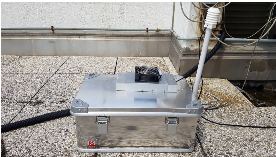
Figure 56 The aluminium box for the Peltier system on the roof of CNR-ISAC in Bologna.
