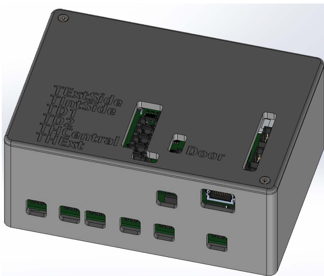
Figure 26 Rendering of the box containing the electronic boards (top view).
